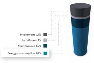
GET THE MOST OUT OF YOUR COMPRESSED AIR Two key elements influencing your system running costs are operating pressure and air leakage. Reducing either can save you considerable amounts of money. Because of the wide pressure band, multiple machine installations operating in a cascade are particularly inefficient. Leaks, on the other hand, have been estimated to waste as much as 30% of
