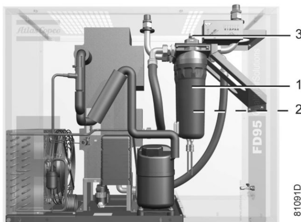
FD 95 with integrated filters option
